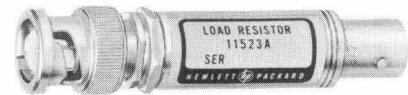
Fig. 5. Optional load resistor is matched to individual detectors for square law conformance within \pm 0.5 db from low level up to 50 mv peak output (at 24°C). Sensitivity of detector with load resistor is typically 0.1 mv/ \mu w.
