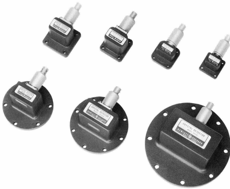
Fig. 4. Series of seven detectors matches waveguide sizes from S through P bands. Diode elements are in sealed capsules, easily replaced without special tools or soldering.
